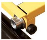
Wheels rest perpendicular on a horizontal steel frame, ensuring the load of the pallet cannot cause misalignment; bumper minimizes load impact.
